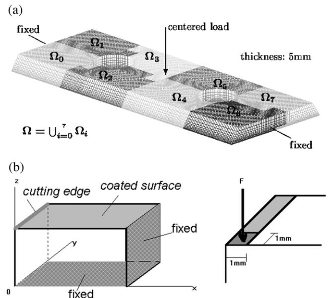
Fig. 1. Domain decomposition of a cutting insert with boundary conditions for a bending simulation (above) and boundary conditions for the simulation of a cutting situation (below).
