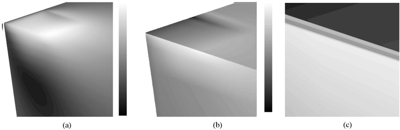
Fig. 5. Computed  $\sigma_{xx}$  for the problem C111Co0 (left) and C111Co3 (middle, right zoomed into the layer region).
