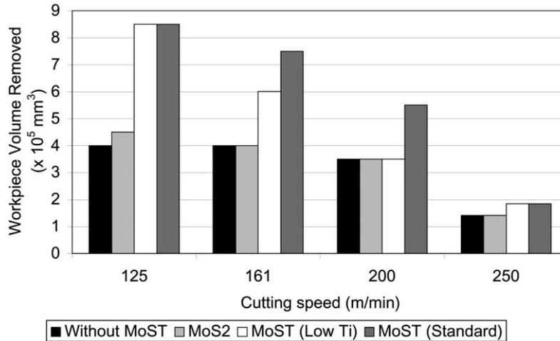
Fig. 13. Dependence of the removed volume of workpiece material up to the end of the tool life of the insert on the cutting speed in milling test. (type 4, 0.25 mm/rev. tooth,  $a_p = 1.5$  mm,  $d = 80$  mm).
