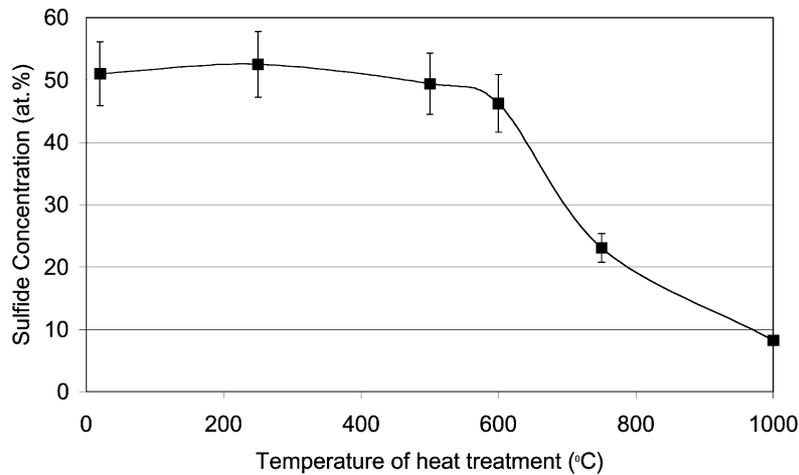
Fig. 5. Dependence of the S concentration of MoS<sub>2</sub>/Ti composite coating [ $X(\text{Ti})=16$  at.%] for as deposited state) on the heat treatment temperature after heat treatment for 1 h in vacuum.
