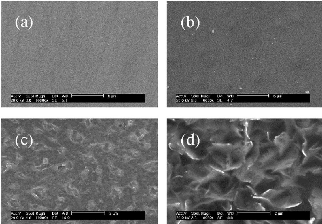
Fig. 4. Surface morphology of MoS<sub>2</sub>/Ti composite coatings [ $X(\text{Ti})=16$  at.%] after heat treatment for 1 h in vacuum. (a) As deposited; (b) at 250 °C; (c) at 500 °C; (d) at 750 °C.
