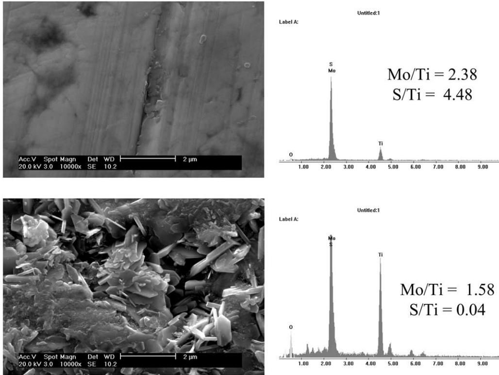
Fig. 11. Surface morphology and its composition of rake surface of MoST coated turning insert (standard condition, after 1 min turning test, type 1). (a) Far from the contact zone with workpiece material and (b) underneath the contact zone with workpiece material.
