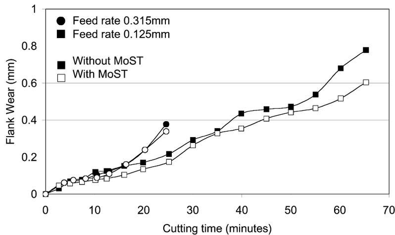
Fig. 12. Summary of dependence of the flank wear of turning inserts on the time of cutting in continuous turning conditions. (type 2) for two different feed rates.
