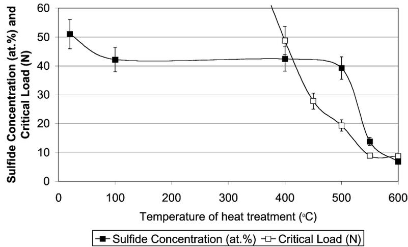
Fig. 8. Dependence of the: (a) S concentration; and (b) the adhesion strength of MoST coating on the oxidation temperature after 10 min oxidation in air.
