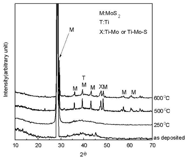
Fig. 3. XRD patterns for MoS<sub>2</sub>/Ti composite coatings [X(Ti)=16 at.%] after heat treatment for 1 h in vacuum.
