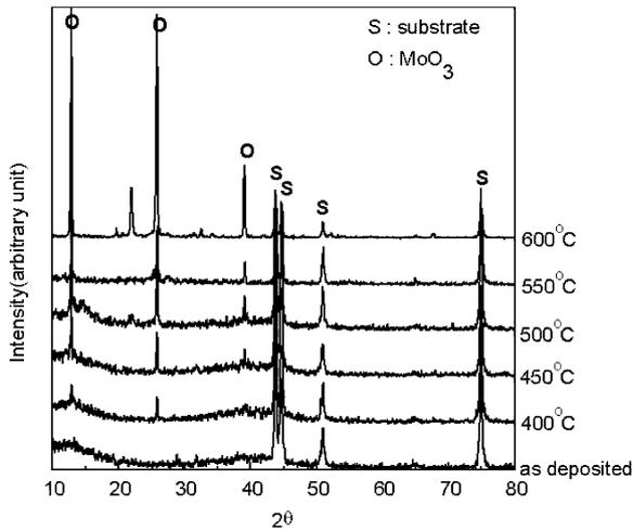
Fig. 6. XRD patterns for  $\text{MoS}_2/\text{Ti}$  composite coatings after oxidation for 10 min in air.
