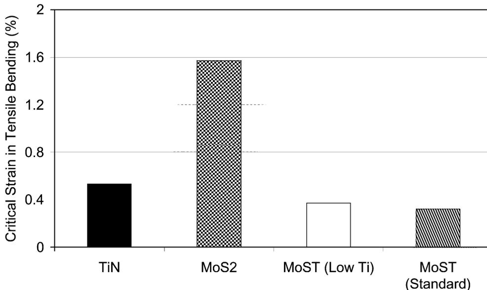
Fig. 1. Comparison of critical strain of TiN, MoS<sub>2</sub> and MoST coatings on SS316 stainless steel as a function of Ti concentration.
