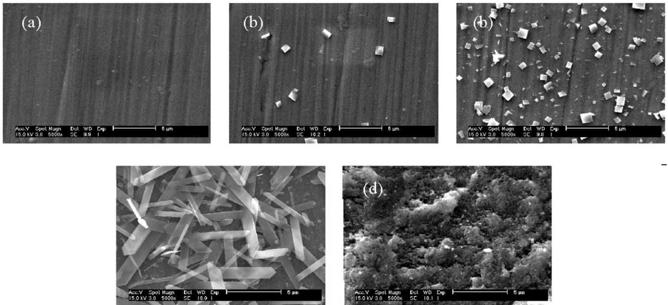
Fig. 7. Surface morphology of  $\text{MoS}_2/\text{Ti}$  composite coatings after oxidation for 10 min in air: (a) as deposited; (b) at 400 °C; (c) at 500 °C; (d) at 550 °C; and (d) at 600 °C.
