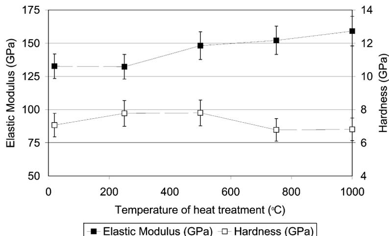
Fig. 2. Dependence of the elastic modulus and the hardness of MoS<sub>2</sub>/Ti composite coatings [X(Ti)=16 at.%] on the heat treatment temperature in vacuum.
