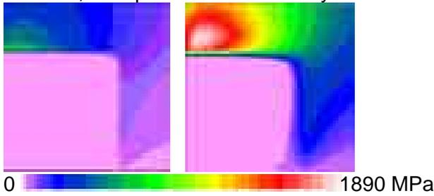
Fig. 17:  $\sigma_{yy}$  below the contact area
